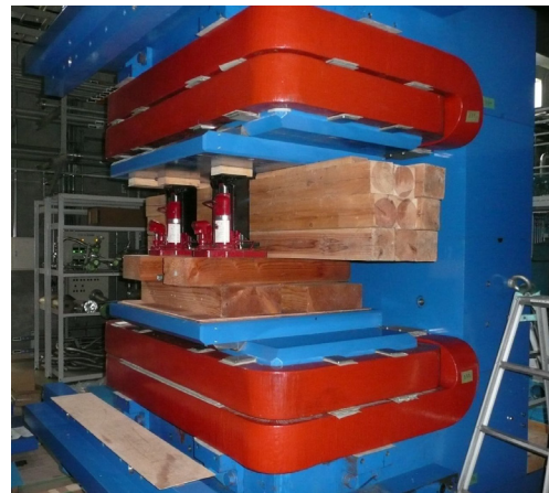
Fig. 17: The Kappa magnet with pole extensions during installation in the NU1 building.
