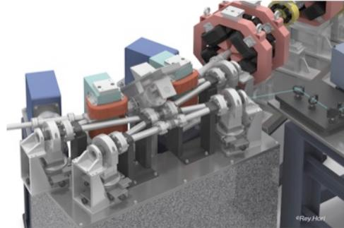
Fig. 6: Illustration of Laser accumulation chamber.
