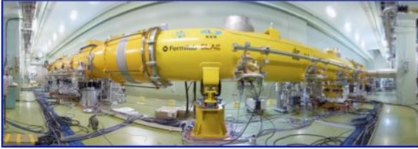
Fig. 1: S1-Global cryomodule experiment setup in STF tunnel. Two cryomodules and the cold box were connected.
