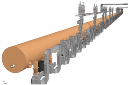
Fig. 9: RF power distribution scheme of TDR.
