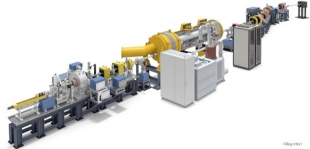
Fig. 3: Installation STF accelerator for use of Quantum Beam experiment.
