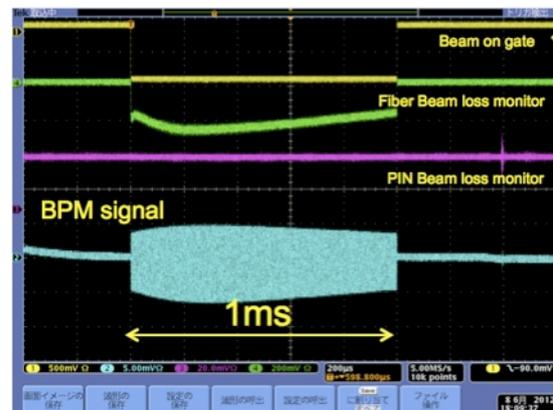
Fig. 7: Scope signal for accelerated 1ms beam train.
