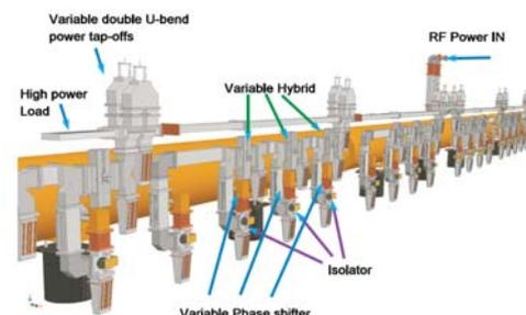
Figure 8: 3D view of Local Power Distribution System
