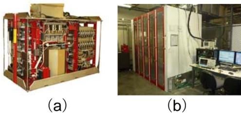
Figure 6: (a) Marx modulator of DTI (b) P2 Marx of SLAC
