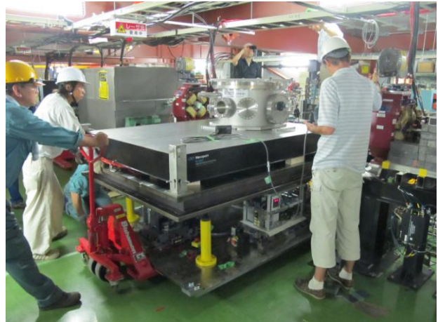
Fig 5: Installation of the four-mirror cavity in ATF.
