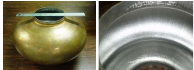
Fig. 5. Seamless cavity (Nb/Cu clad) left: inside of the cavity
