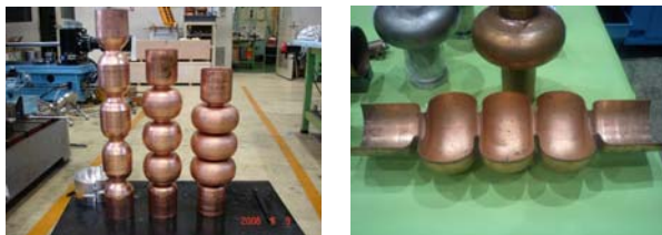
Fig. 1. Seamless three-cell cavities made by necking and hydroforming (test modules made of copper).
