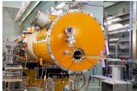
Figure 1: Cryomodule performance test with magnetic field measurement.
