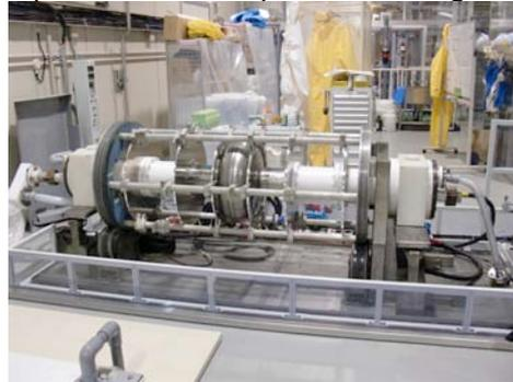
Fig. 4: Second EP system for KEKB cavities, ERL, and ILC cavities.
