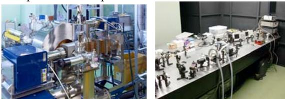
Fig. 8: Assembled photocathode RF gun system (left) and drive laser system (right) for beam source of Phase-2.
