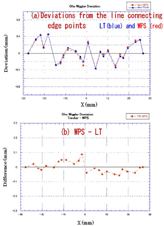
Figure 6: Comparison between WPS and Blue tracker measurements of positions of holes for alignment target insertion on the KEKB wiggler magnets. (a) Deviations of each measurement from the line connected both edge points for WPS (red) and Blue tracker (blue). (b) Differences between WPS measurement and Blue tracker measurement.
