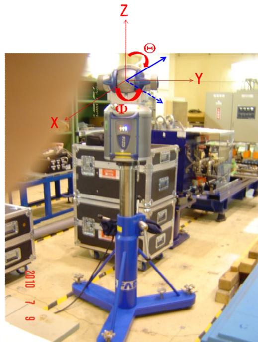
Figure 1: Picture of a FARO Laser Tracker. Definition of the coordinate system is shown in the figure.
