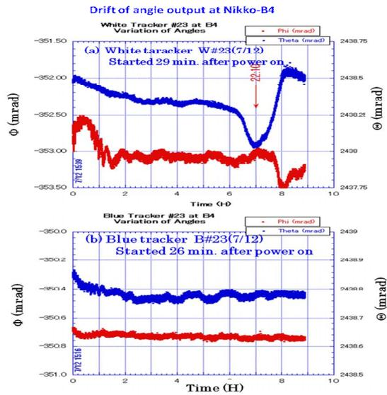
Figure 3: Drift of horizontal angle ( $\Phi$ , red plot) and vertical angle ( $\Theta$ , blue plot) for (a) White tracker and (b) for Blue tracker.
