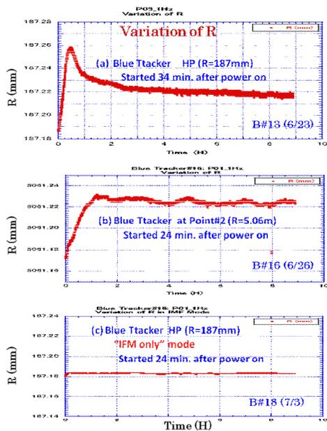
Figure 2: Drift of R (distance) data after machine ready (a) at HP (Home Position), (b) at a point about 5m far, and (c) drift in case of IFM (InterFerometer Mode).
