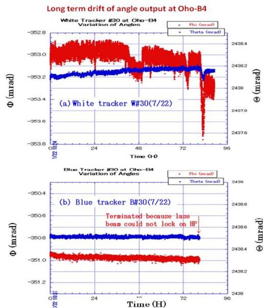
Figure 4: Long term variation of horizontal angle ( $\Phi$ , red plot) and vertical angle ( $\Theta$ , blue plot) (a) for White tracker and (b) for Blue tracker.
