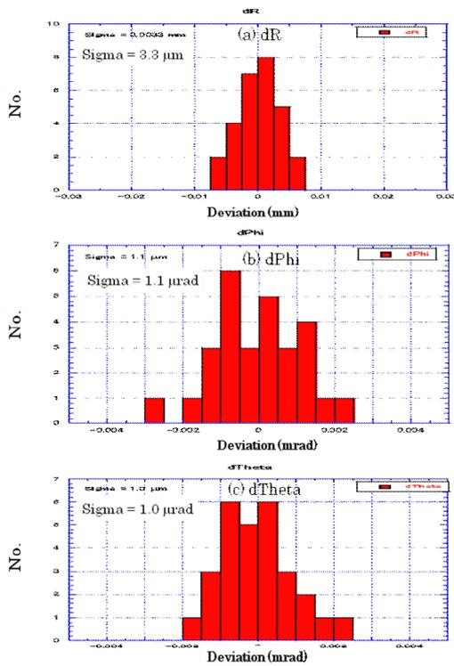
Figure 5: Histograms for RMS for measurement at each monument, (a) for R, (b) for  $\Phi$  and (c) for  $\Theta$ .
