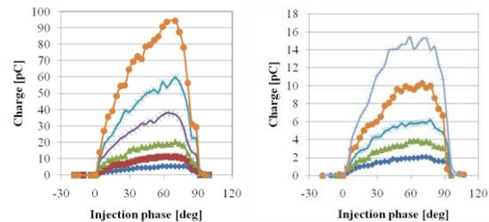
Figure 2: Bunch charge as a function of injection phase of the femtosecond UV light. In the left figure, the UV spot size and power were 2 mm  $\phi$  and ranging from 1 to 15  $\mu\text{J}/\text{pulse}$ . In the right figure, the UV spot size and power were 2 mm  $\phi$  and ranging from 0.5 to 4  $\mu\text{J}/\text{pulse}$ .
