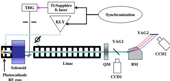
Figure 1: Schematic diagram of a femtosecond electron source.
