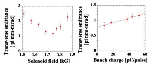
Figure 3: Emittance at the linac exit as a function of magnetic field of the solenoid (left). The laser injection phase and the bunch charge were  $25^\circ$  and 50 pC/pulse,
