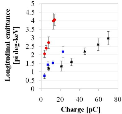
Figure 5: Longitudinal emittance as a function of bunch charge. The red, blue and black plots indicate the laser spot diameter on the cathode of 0.5, 1, 2 mm, respectively.
