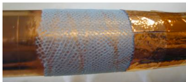
Fig. 11 Polyethylene mesh as a spacer.
