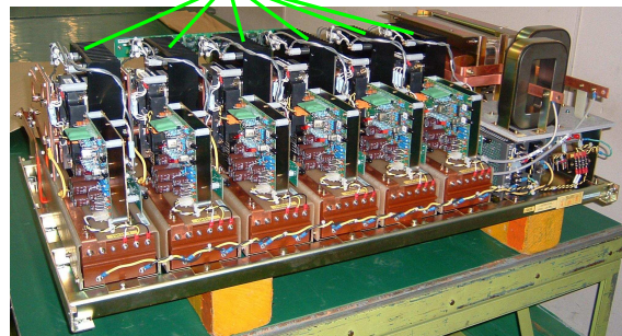
Figure 4: External appearance of the IGBT switch unit.
