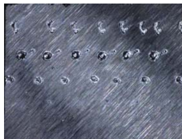
Fig. 11 Mo surface shot by EBW at KEK.
