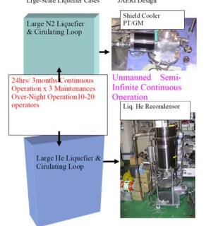
Figure 2 : Comparison between large-scale liquefier and Zero-boil off refrigerator
