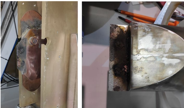
Figure 4: Broken part of the circulator port-1 (2022/Jan).
