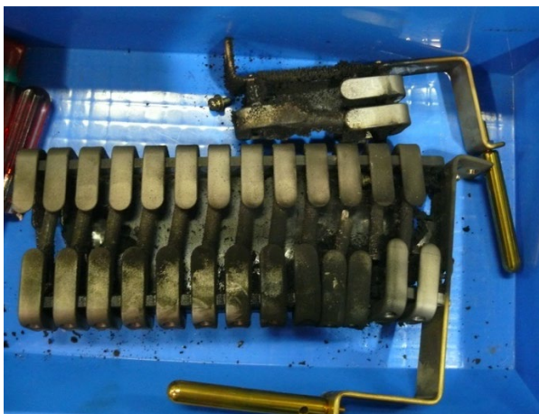
Figure 5: Discharge on the surface of Schenkel column (high energy side column). Such discharge by-passes some rectifier circuits, which act as damping resistors for the resonance circuit of RF coil and RF electrodes (top). Q-factor decreases and resonance current increases. Finally, over current error is activated and trip the RF driver. Sometimes before trip of RF driver, the shorten circuits are burned out (middle and bottom).
