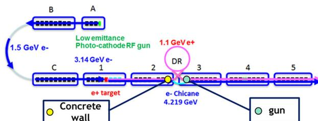
Figure 1: Schematic layout of the SuperKEKB injector Linac.
