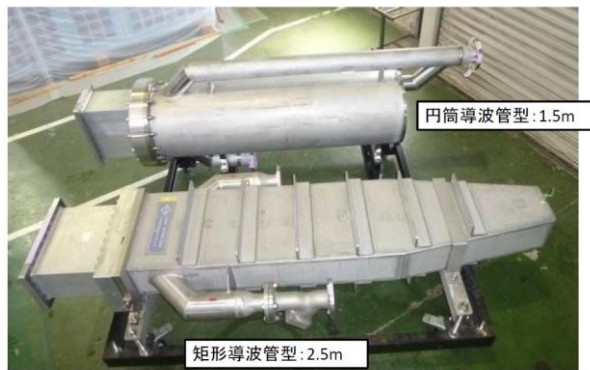
Figure 4: High power water-loads.
