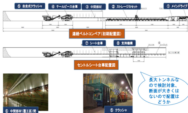
Figure 13: Continuous belt conveyor system for mucking.
