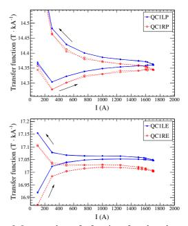
Figure 5: Integrated transfer function of quadrupole term at different current level in steady-state. Top: QC1LP (solid curve) and QC1RP ( dashed curve ). Bottom: QC1LE (solid curve) and QC1RE ( dashed curve ).
