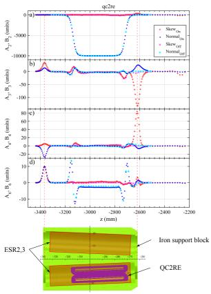
Figure 8: The axial profiles of QC2RE quadrupole magnet. The iron support block is indicated at a same scale and position in the axial direction.
