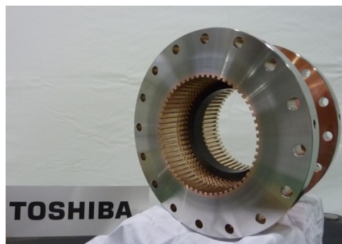
Figure 1: A completed prototype HOM absorber.
