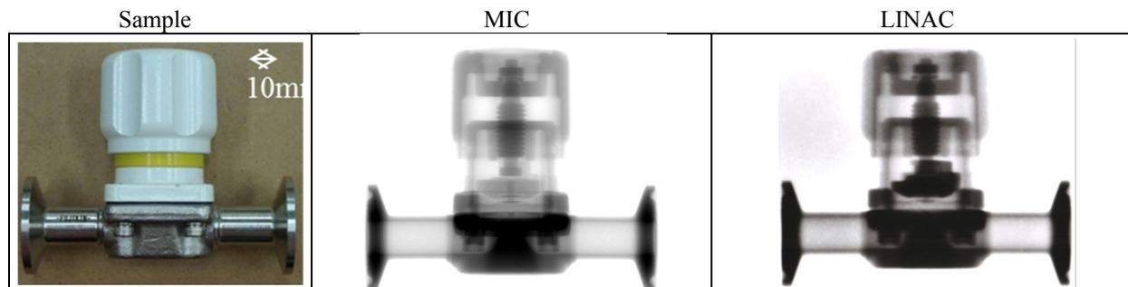
Figure 11: Difference in imaging between MIC and LINAC are shown. Because the focal spot size is smaller with MIC, the image of MIC has less blur than with LINAC, and image is clearer.
