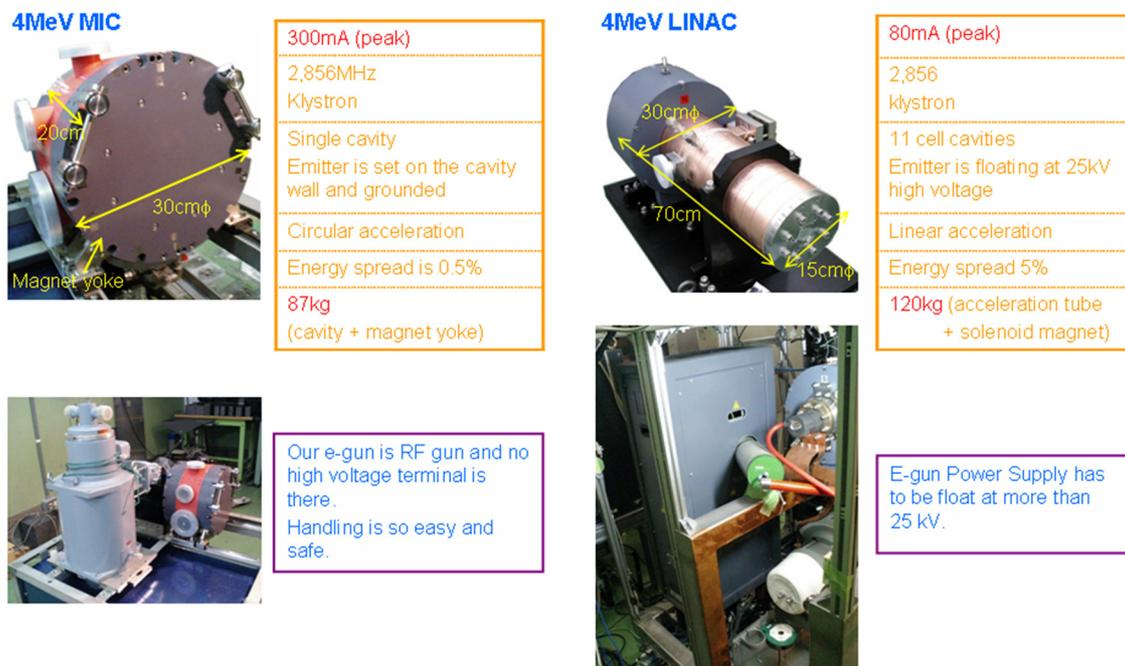
Figure 10: Differences in hard ware are shown between MIC (left) and LINAC (right).
