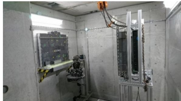
Figure 2: X-ray CT manipulator and flat panel 2D Detector (FP) are seen in the 1m thick concrete shielding room. Maximum 70 kg object is acceptable on the manipulator. FP size is 40 x 40 cm<sup>2</sup> with 200  $\mu\text{m}$  pixel.
