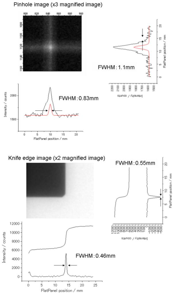
Figure 5: MIC beam spot size is measured by pinhole (top) for MIC1 and by knife edge (bottom) for MIC6.
