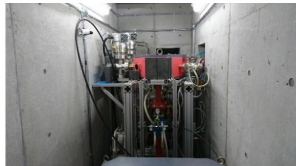
Figure 3: MIC6 is used for advanced X-ray CT non-destructive testing. Electron focal spot size 0.25 mm is achieved for X-ray imaging.
