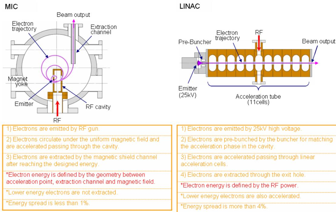
Figure 9: Differences in acceleration mechanism are shown between MIC (left) and LINAC (right).
