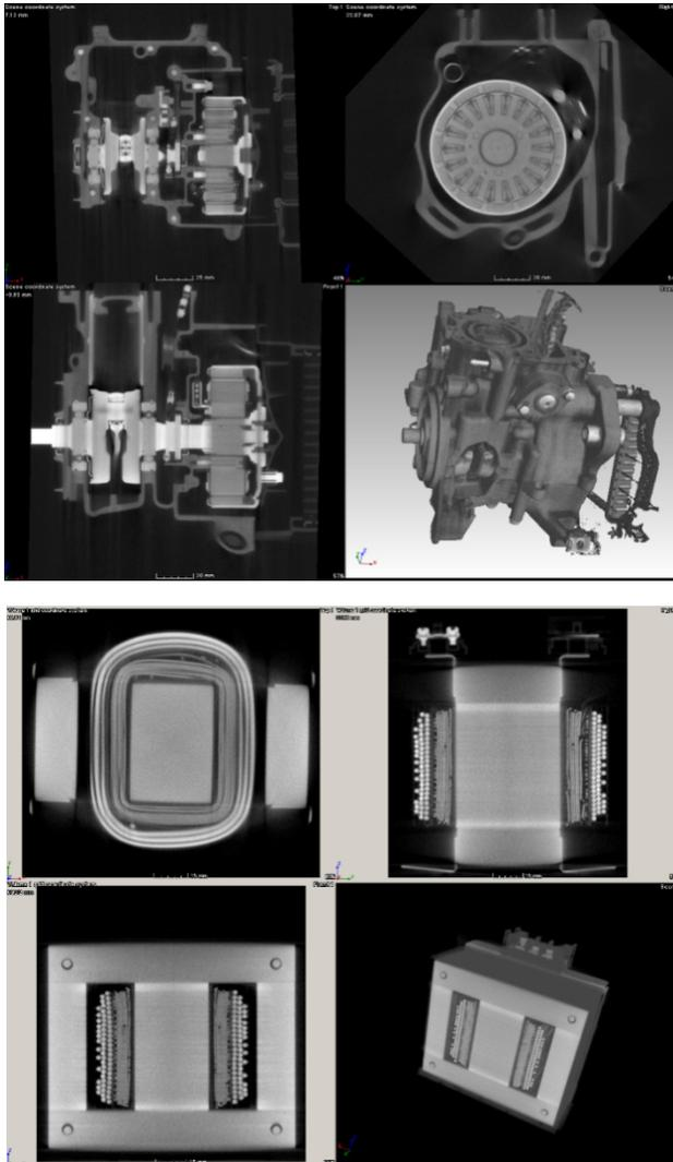
Figure 4: Top is cross sections of a motor engine. Bottom is a 30cm wide trans.
