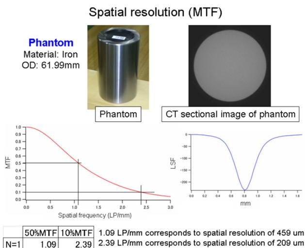
Figure 6: MTF inspection of CT resolution taken by standard phantom 61.99 mm wide iron rod.
