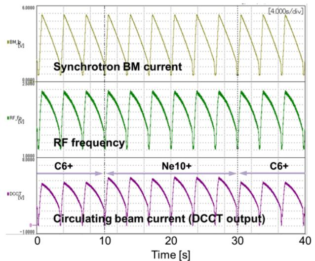
Figure 4: Operation test of multi-ion acceleration switching ion species of injection beams between  $^{12}\text{C}^{6+}$  and  $^{20}\text{Ne}^{10+}$ .
