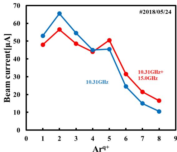
Figure 5: Charge state distributions of argon. Comparison between single heating (10.31 GHz) and two heating (10.31 + 15.0 GHz).
