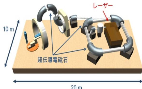
Figure 2: Quantum scalpel including a laser injector a compact superconducting synchrotron and a compact superconducting gantry.
