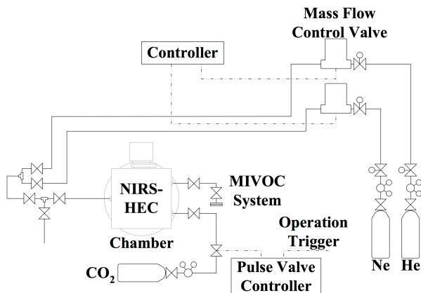
Figure 6: Gas-pulsing system for multi-ion production.
