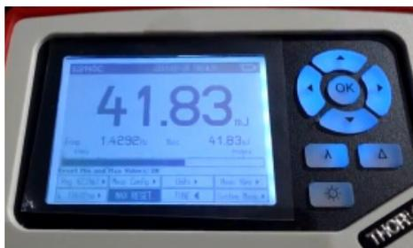
Figure 2: The maximum macro-pulse energy available at the user station #1. This was recorded after a user experiment on 28th July, 2018.
