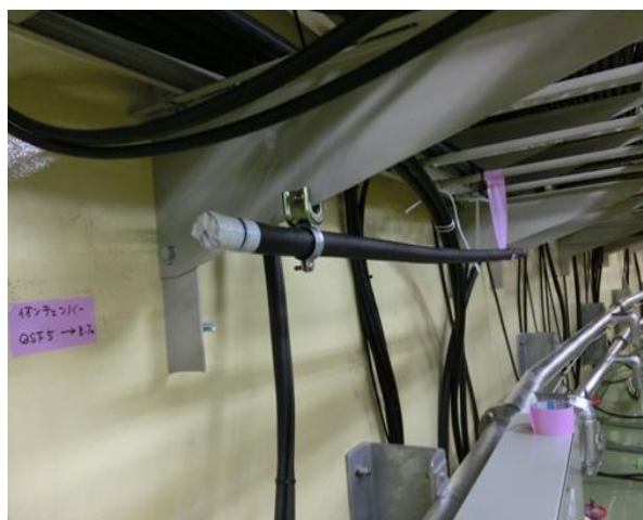
Figure 6: Ion chamber for the beam loss monitor.
