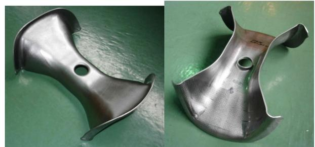
Figure 5: Press formed shape after burring with niobium sheet of 2.5 mm thick.
