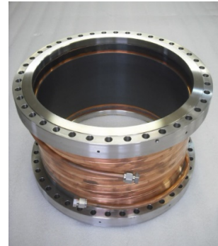
Figure 4: A KEKB type LBP damper with 4-mm thickness of ferrite, \phi 300 mm, length of 150 mm.
