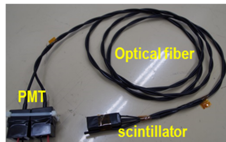
Figure 5: Photograph of an optical fiber beam loss monitor.
