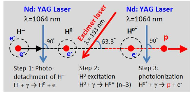
Figure 3: Schematic view of principle for H<sup>-</sup> stripping to proton by using only lasers. Noted parameters are typical ones estimated for the 400 MeV H<sup>-</sup> beam energy.
