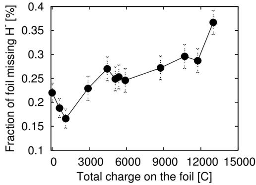
Figure 2: Measured unstripped H<sup>-</sup> as a function of charge via the foil during beam operation. The missing H<sup>-</sup> was increased nearly 3 times higher as compared to that in the beginning of the operation. Such an increase of the waste beam may limits the foil lifetime at 1 MW operation.
