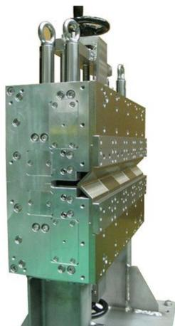
Figure 3: Prototype of the DC septum.
