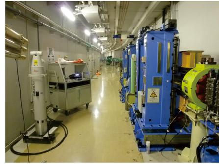
Figure 3: Leica SMART310 laser tracker.
