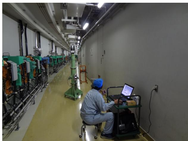
Figure 6: Horizontal coordinate measurements with Leica AT402 laser tracker.
