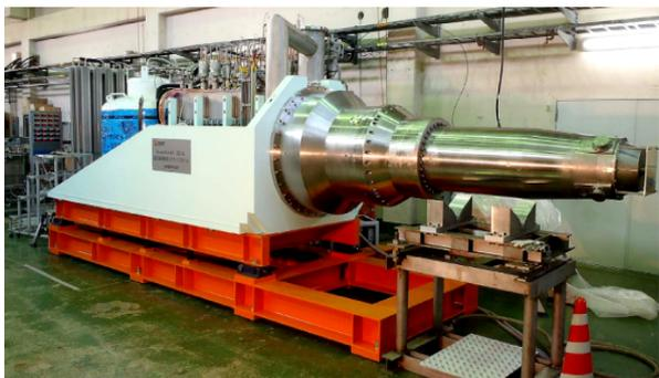
Figure 2: The QCS-L cryostat in the KEK laboratory.
