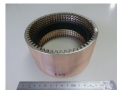
Figure 1: Test piece of brazing.
