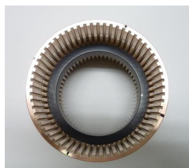
Figure 7: AIN/Cu cylinder after brazing.
