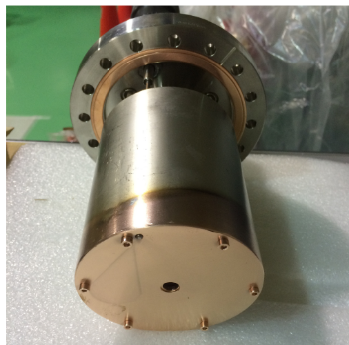
Figure 6: Photograph of the Four-Grid analyzer for the IFMIF/EVEDA prototype accelerator.
