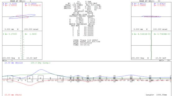
Figure 3: Matching design of the DTL using TRACE3D.
