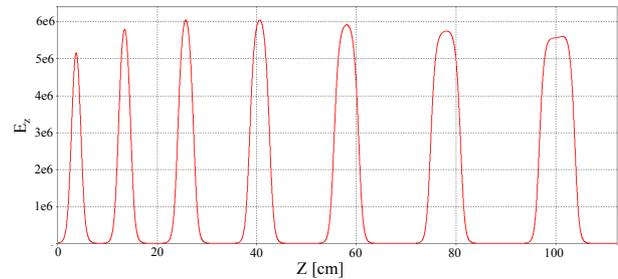
Figure 5: Longitudinal electric-field profile along the cavity.
