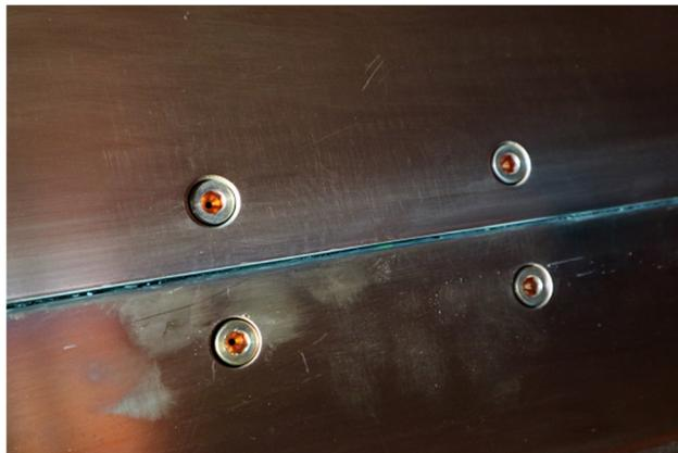
Figure 1: Interspace between flanges of fRC RF-W Cavity.
