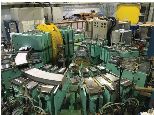
Figure 5: The ERIT ring is now under modification. Additional poles have been installed in order to modify the  $k$  value suitable to demonstrate the serpentine accelerations and the extended ERIT mechanism.
