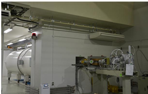
Figure 2: Photo of an accelerator and a beam transport line.
