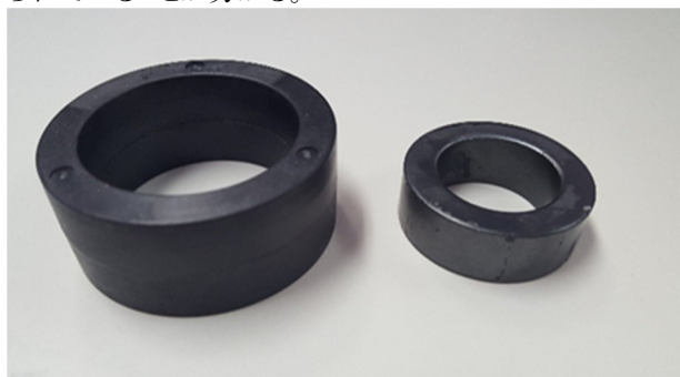
Figure 2: FINEMET and 43 Material core.
