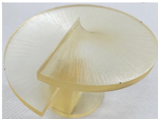
Figure 5: Helical target for electron penetration depth measurement into water.
