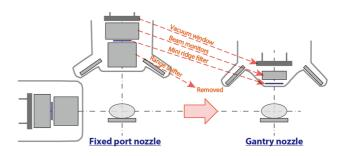
Figure 6: Comparison of nozzle design between fixed port and gantry port.
