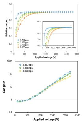
Figure 8: Example of beam monitors test result. Upper is recombination measurement of dose monitor, lower is gain measurement of beam position monitor.
