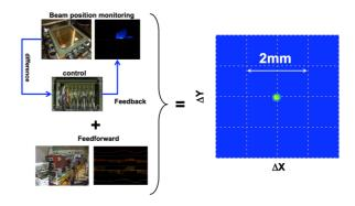
Figure 3: Feed-forward and feed-back control for precise control of scanned ion beam.
