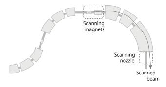
Figure 5: Layout of scanning system on rotating gantry.
