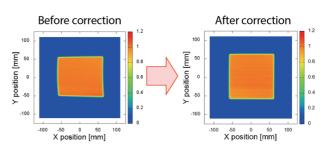
Figure 9: Correction of scanned beam distortion.
