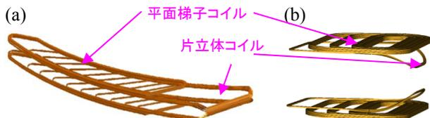
Figure 1: Schematic views of the Spiral FFAG magnet. (a) Designed coil shape for practical use. (b) Coil of the model magnet to implement coil winding technology.
