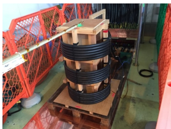
Figure 4: Dummy load(MLFC: 250 mm 2 , Diameter 600 mm/6 Turns×3 circuits=18 Turns).
