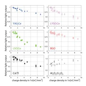
Figure 6: Charge density and relative output of the luminescence. The light output is normalized by the light output of the maximum beamsize point.
