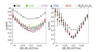
Figure 5: Comparison of electron beam sizes measured with different scintillating screes. The left and right figure show the horizontal and the vertical beam size as a function of the quadrupole strength, respectively. Error bars represent RMS for 10 times measurement of the beam size.
