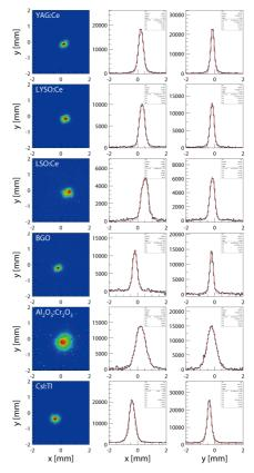
Figure 4: Background corrected beam images and profiles measured with different scintillating screens.
