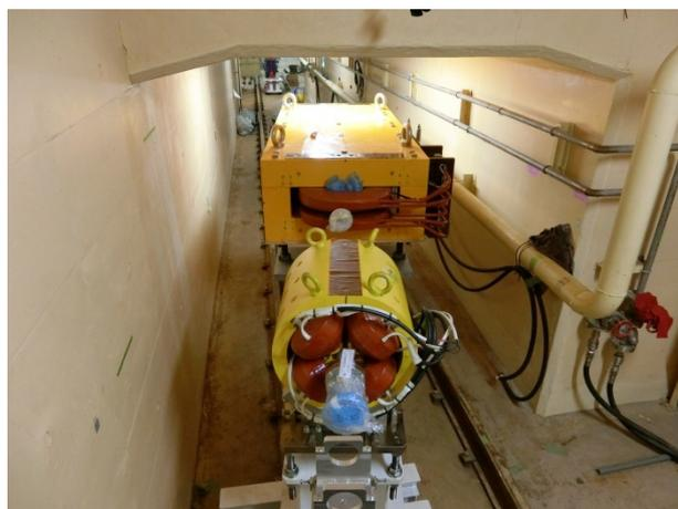
Figure 8: A Bending magnet and a quadrupole magnet at the SY3 beam dump tunnel.
