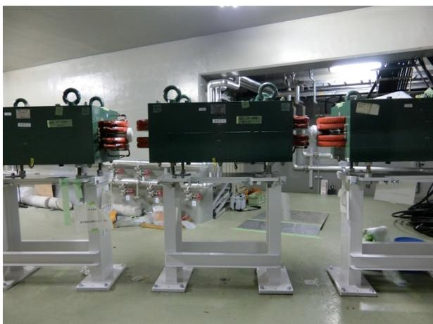
Figure 6: The Bending magnets and the vacuum chambers at matching section.
