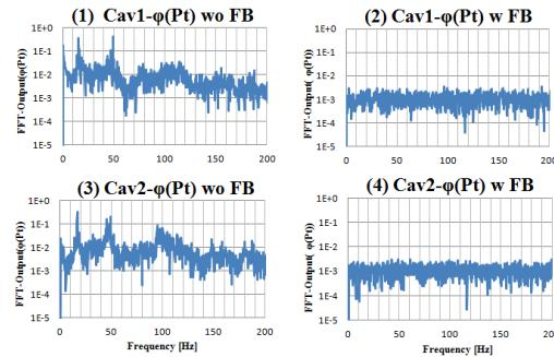
Figure 1: Microphonics on 9-cell cavities. There are 15.4Hz and 49.3Hz as the components in Cavity#1, and 16.9Hz, 45.6Hz, 49.3Hz as well as 100Hz in Cavity#2. When the feedback function on LLRF system is turned on, the fluctuations of the the RF phases and the accelerating voltages are suppressed.
