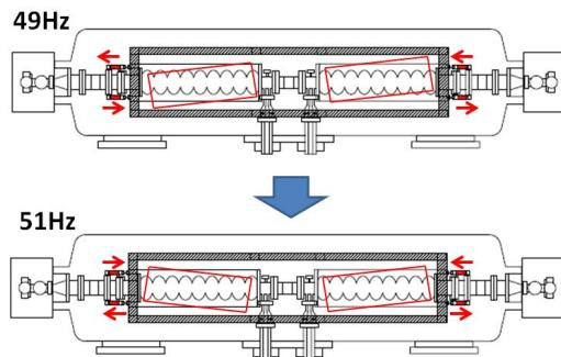
Figure 13: Vibration mode of 49.5Hz. The phase relation among the three piezoes can be summarized to the phase relation among the four piezoes, we can know the directions of the force on the four piezoes.
