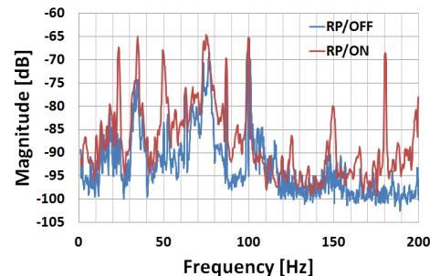
Figure 9: Vibrational state of floor around Main Linac. When the rotary pump turn on, 50Hz component is excited.
