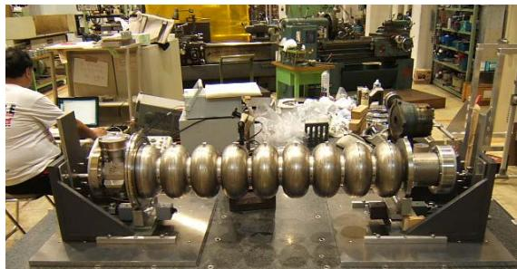
Figure 2: 9-cell cavity on testing. The eigen frequencies of a 9-cell cavity was investigated by forced oscillation technique. Aluminum cubes were put on the top of the equator of each cells, and the amplitudes of X, Y and Z were measured by a capacitive distance meter(MicroSense4830).
