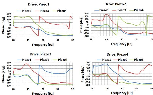
Figure 12: 4 piezoes. There are same phase and opposite phase among three piezoes for 49Hz and 51Hz for either measurement. When the resonance transits from 49Hz to 51Hz, those phase condition changes, too. It is thought that 49Hz and 51Hz are different vibration modes.
