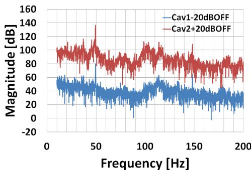
Figure 7: Fluctuation of RF signal. It shows only the 50Hz fluctuation seen in LLRF. It is unknown why the 15Hz peak does not appear.
