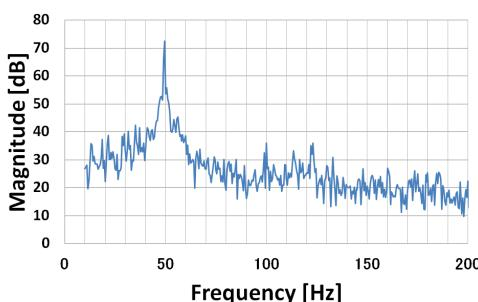
Figure 8: Results of RF free run. The output signal of piezo element was directly input to FFT analizer. It shows only 50Hz resonant as same as previous RF measurement.
