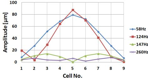
Figure 3: Resonant mode of 9-cell cavity. It shows the eigen vibration of the 9-cell cavity. 58Hz, 147Hz and 260Hz are the fundamental wave, the two times and the three times wave of the transverse wave, 124Hz is the fundamental wave of the longitudinal wave.
