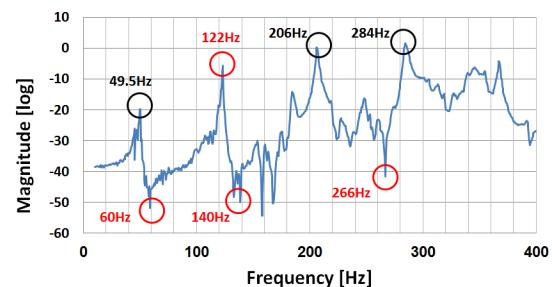
Figure 5: Result of piezo to piezo test. The resonances with red circle are as same as Figure 3.
