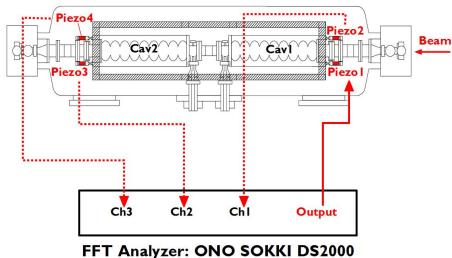
Figure 11: Phase measurements among 4 piezoes. A multi-channel FFT analyzer is used. One piezo was used as the drive oscillator of forced oscillation technique, and the phase relations among three piezoes were confirmed. The drive piezo was cyclically changed.
