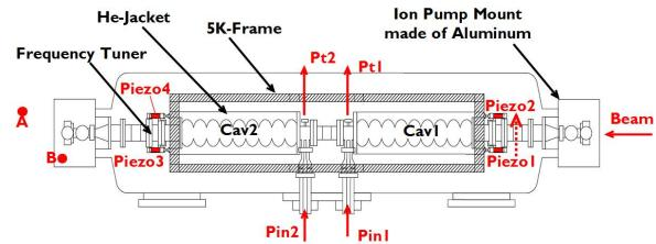
Figure 4: Composition of main linac on cERL. The cryomodule of Main Linac includes two 9-cell cavities mounted on the 5K-frame. Each cavity has two piezo elements as frequency tuner, and using these piezo elements, forced oscillation technique was carried out.
