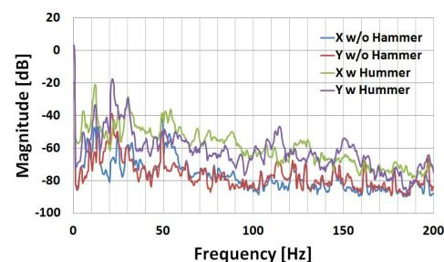
Figure 10: Vibrational state of cryomodule. Using hammer in order to excite the eigen vibrations of the cryomodule, vibration of frequency range less than 50Hz was excited. This vibration is possible to contribute the microphonics, 15Hz and 50Hz.
