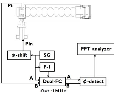
Figure 6: Setup of RF measurement. When Main Linac was cooled down at 2K, the RF fluctuations of two 9-cell cavities were measured by phase difference between Pin and Pt.
