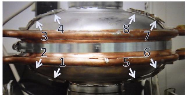
Figure 2: Thickness measurement points on the cell.
