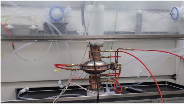
Figure 7: Improved tap water cooling.
