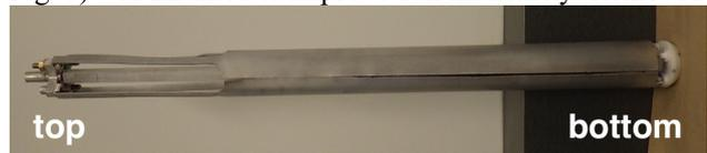
Figure 3: Thicker rod cathode.
