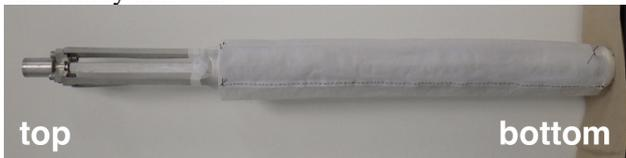
Figure 4: Rod cathode covered with cathode bag.
