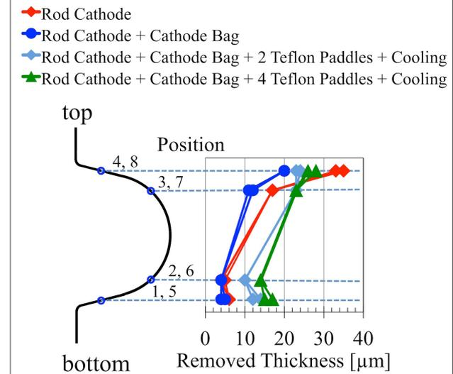
Figure 9: The results show the tendency that upper area is etched more. Paddles and cooling resulted more uniform etching.
