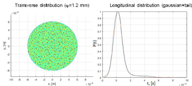
Figure 4: Input distribution simulated at the cathode.
