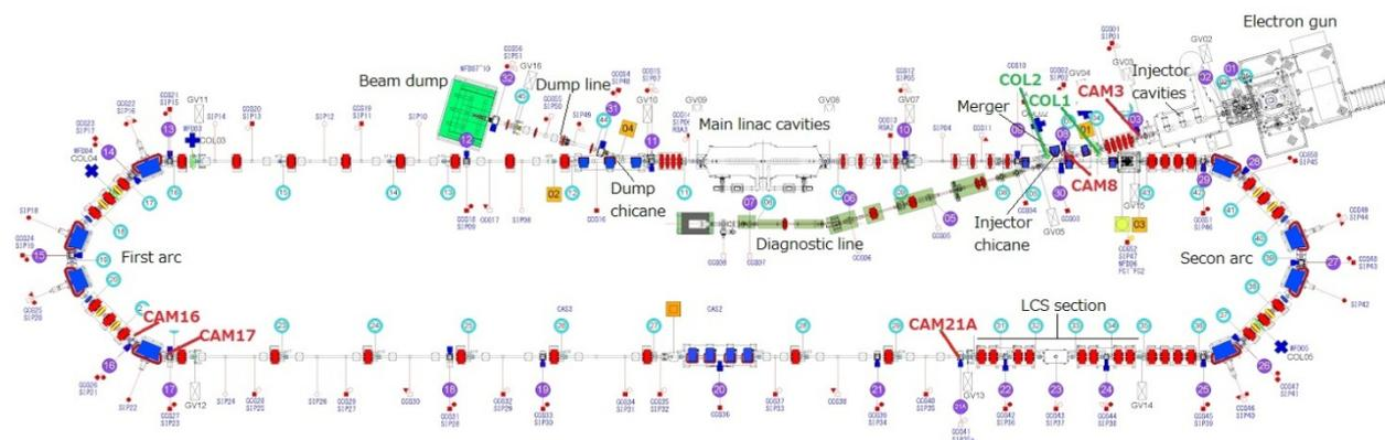
Figure 1: Layout of cERL with measurement equipment.
