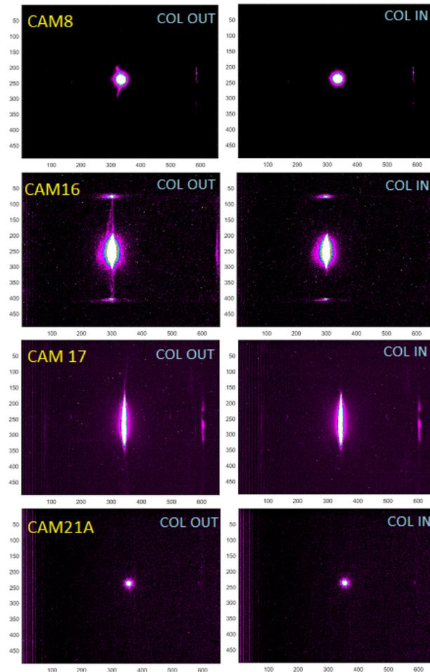
Figure 2: Observed vertical beam halos. CAM8: 3/2, burst mode, gain 22, integration time 10  $\mu$ s, CAM16 – 17: 3/9, long pulse mode, gain 22, integration time 2 ms, CAM21A: 3/14, burst mode, gain 22, integration time 10  $\mu$ s.
