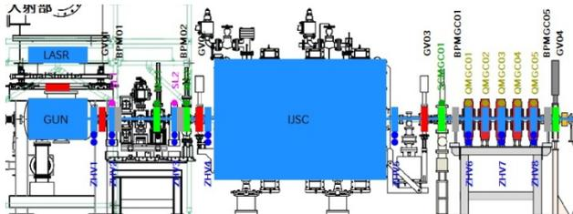
Figure 3: Layout cERL of injector line.
