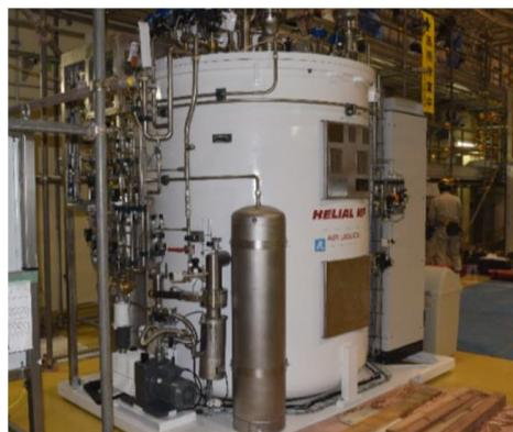
Figure 12: Cold box for cryoplant.
