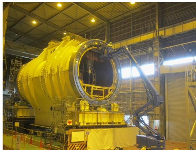
Figure 6: Rotation tests of the gantry structure at the Toshiba Keihin Product Operations.
