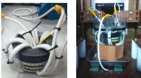
Figure 7: (Left) another prototype balun, (right) it is dipped in fluorinert.
