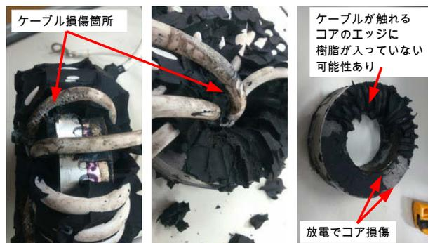
Figure 6: The balun was broken by the discharge inside.
