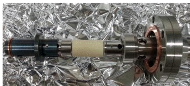
Figure 3: Photograph of the cathode plug and mount of the cathode. The cathode plug is electrically isolated from the vacuum chamber to enable measurement of photo-induced current and quantum efficiency of the cathode.
